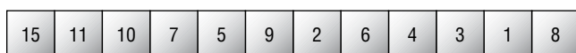
Figure 10.5: You can store a heap, or any complete binary tree, conveniently in an array.
